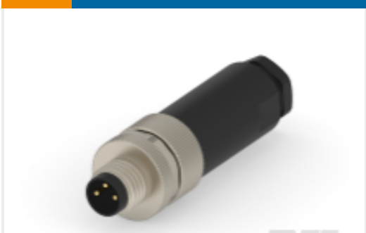
TE Part # T4011008031-000 M8,SCREW, MALE,S,UNSHIELD,3P, GOLD
