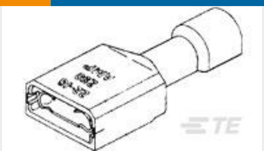
TE Part # 2-520261-2 ULTRA-FAST 187 ASY REC 22-18 TPBR
