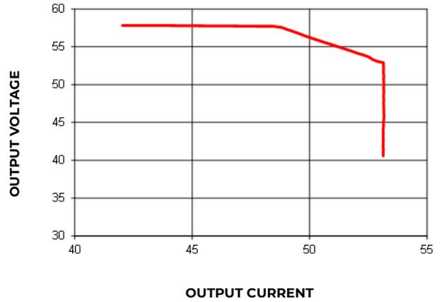
Figure 2. 54V<sub>DC</sub> output: Power limit, Current limit and shutdown profile at  $V_{IN} = 185V_{AC}$
