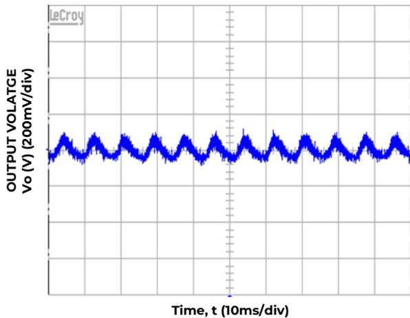
Figure 5. 54V<sub>DC</sub> output ripple and noise, full load,  $V_{IN} = 185V_{AC}$ .
