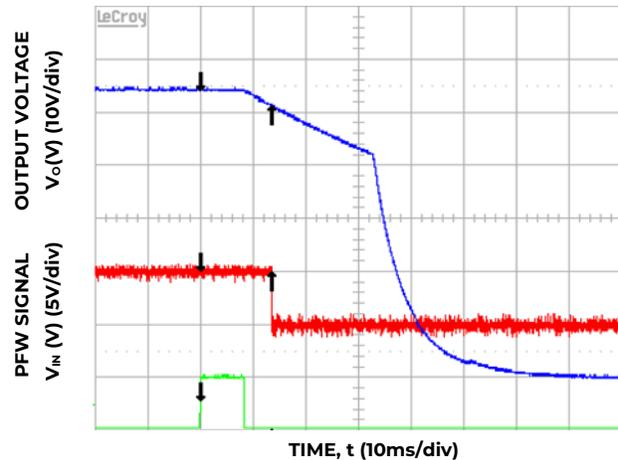
**Figure 12. PFW alarmed 19.6ms prior to Vo < 40V,
