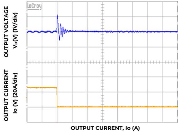
**Figure 8. Transient response 54V<sub>DC</sub> load step
