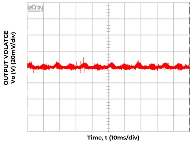
Figure 6. 5V<sub>DC</sub> output ripple and noise, all full load,  $V_{IN} = 185V_{AC}$ .
