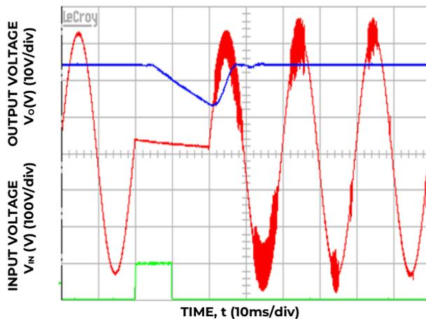
**Figure 11. Ride through missing 1 cycle, full load, V<sub>IN</sub> = 230V<sub>AC</sub>**
