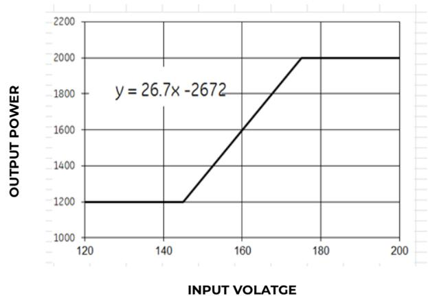
Figure 4. 54V<sub>DC</sub> output: Output power derating based on input voltage.
