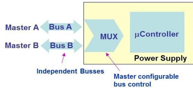
**Figure 14. Diagram showing conceptual representation of the dual I<sup>2</sup>C bus system.**
