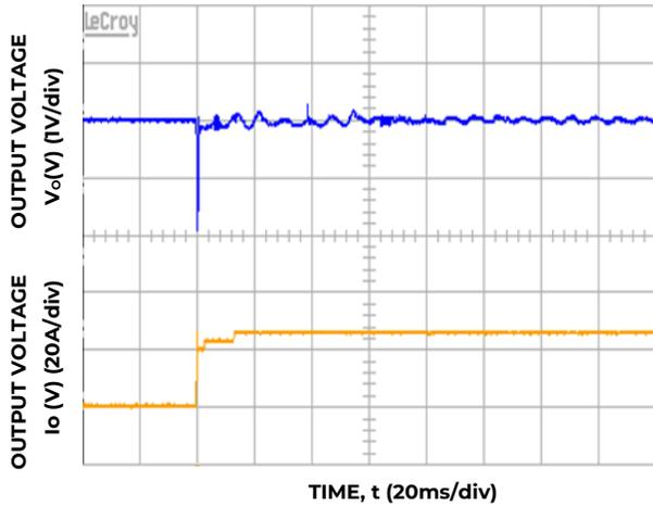
**Figure 7. Transient response 54V<sub>DC</sub> load step
