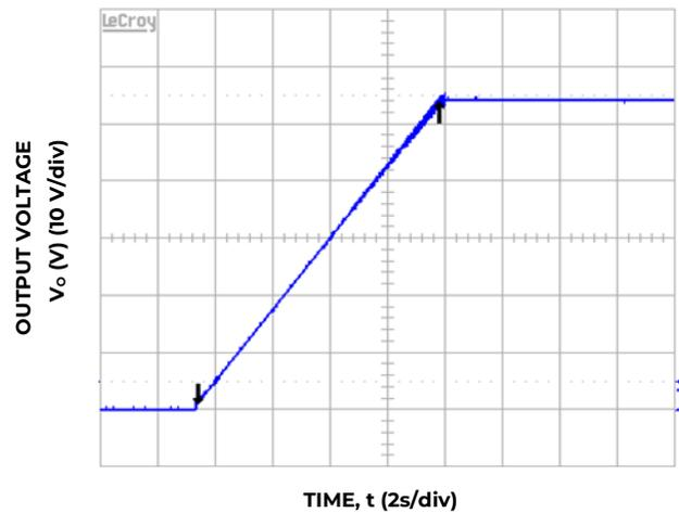
**Figure 10. 54V<sub>DC</sub> soft start, full load,
