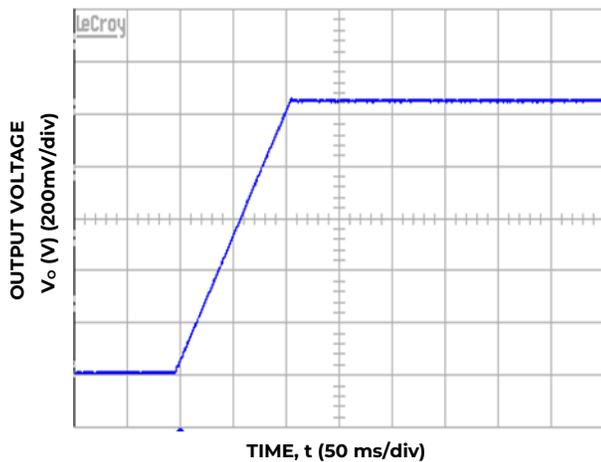
**Figure 9. 54V<sub>DC</sub> soft start, no-load & full load,
