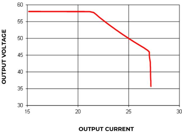
Figure 3. 54V<sub>DC</sub> output: Power limit, Current limit and shutdown profile at  $V_{IN} = 90V_{AC}$ .
