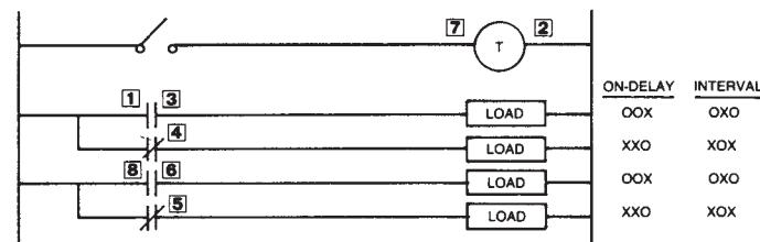
\*For Interval Operation with a Momentary Start Switch, Jumper 7 & 3
