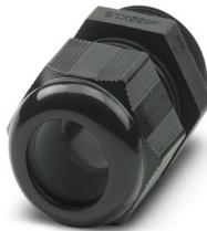
Cable gland, material for screw connection: PA, application: Standard, external cable diameter 15 mm ... 21 mm, shielding: no, connecting thread: M32 x 1.5, color: jet black RAL 9005
