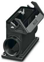
Box mounting bases B24, with single locking latch, material: PA, cable outlets: 2, lateral, 2x M32, height: 84 mm, cable gland: none, Standard, including 2x reducing adapter
