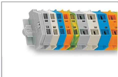
Terminal strip with mounting flanges, for screw or similar mounting types, 3.2 mm mounting hole diameter (with 209-123 Mounting Foot also for DIN-35 rail)
