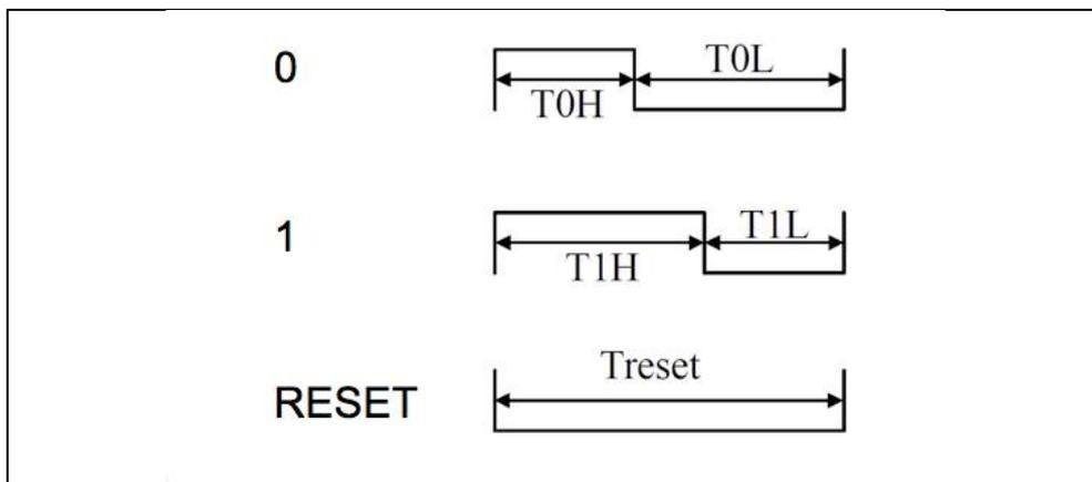
2. The data transmission time ( $T_H+T_L=1.25\mu s\pm 600ns$ ):
