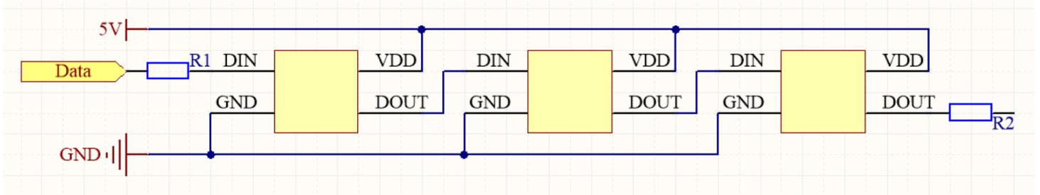
Product signal input and output must be connected in series with protection resistor R1. R1 depends on the size of the cascade amount, the greater the number of cascade, the smaller R1. The general recommended value is between 200-2K $\Omega$ , usually the recommended value is typical 500 $\Omega$ .
