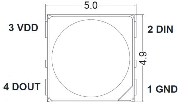
**Figure 2. IN- PI55QATPRPGPBPW-XX Pin Configuration**
