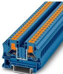
Feed-through terminal block, nom. voltage: 1000 V, nominal current: 41 A, number of connections: 2, number of positions: 1, connection method: Push-in connection, Rated cross section: 6 mm<sup>2</sup>, cross section: 0.5 mm<sup>2</sup> - 10 mm<sup>2</sup>, mounting type: NS 35/7,5, NS 35/15, color: blue
