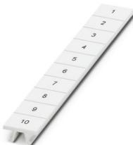
Zack marker strip, Strip, white, labeled, can be labeled with: CMS-P1-PLOTTER, Printed vertically: consecutive numbers 1 ... 10, 11 ... 20, etc. up to 91 ... 100, mounting type: snapped, for terminal block width: 8.2 mm, lettering field size: 10. 5 x 8.15 mm, Number of individual labels: 10
