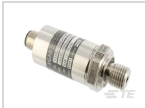
Pressure Sensor Type: **Industrial Pressure Transducer**Pressure: **14 bar [ 203.05 psi ]**Pressure Type: **Absolute**Supply Voltage Range: **9 - 30 V**Output Signal Type: **4 - 20 mA**
