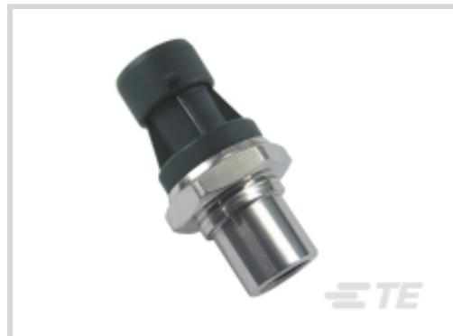
Pressure Sensor Type: **Industrial Pressure Transducer**Pressure: **2 bar [ 29 psi ]**Pressure Type: **Absolute**Supply Voltage Range: **4.75 - 5.25 V**Output Signal Type: **.5 - 4.5 V**
