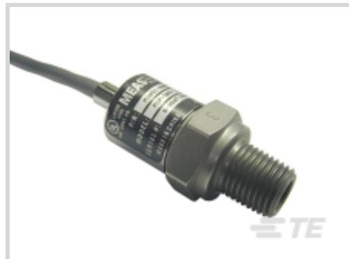
Pressure Sensor Type: **Industrial Pressure Transducer**Pressure: **7 bar [ 101.52 psi ]**Pressure Type: **Gauge**Supply Voltage Range: **5 V**Output Signal Type: **0 - 100 mV**
