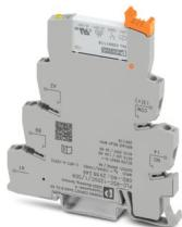
PLC-INTERFACE for input functions, consisting of PLC-BSC.../SEN basic terminal block with screw connection and plug-in miniature relay with power contact, for mounting on DIN rail NS 35/7,5, 1 N/O contact, input voltage 120 V AC/110 DC
