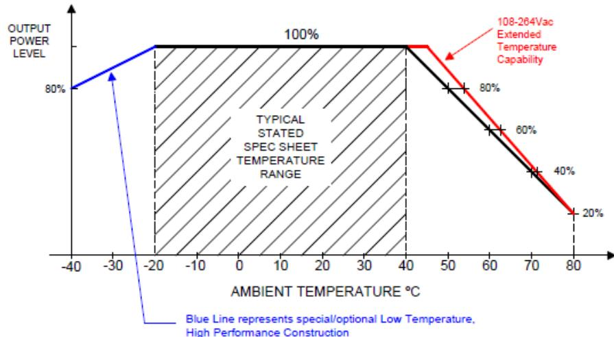
+74C operation with an output power of 19.2W; and cold start at -40C
