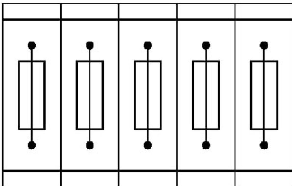
Fuse terminal blocks in interconnected arrangement,
