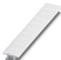
Marker for terminal blocks, Strip, white, labeled, can be labeled with: CMS-P1-PLOTTER, printed horizontally: U, V, W, N, GND, U, V, W, N, GND, mounting type: snapped, for terminal block width: 6.2 mm, lettering field size: 6.15 x 10.5 mm, Number of individual labels: 10
