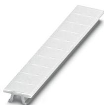
Zack marker strip, Strip, white, unlabeled, can be labeled with: PLOTMARK, CMS-P1-PLOTTER, mounting type: snapped, for terminal block width: 6.2 mm, lettering field size: 6.15 x 10.5 mm, Number of individual labels: 10
