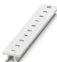
Zack marker strip, Strip, white, labeled, can be labeled with: CMS-P1-PLOTTER, printed horizontally: consecutive numbers 1 ... 10, 11 ... 20, etc. up to 491 ... 500, mounting type: snapped, for terminal block width: 6.2 mm, lettering field size: 6.15 x 10.5 mm, Number of individual labels: 10
