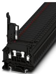
Fuse modular terminal block, fuse type: Glass / ceramics / ..., fuse type: G / 5 x 20, nom. voltage: 60 V, nominal current: 6.3 A, number of positions: 1, connection method: Screw connection, Rated cross section: 1.5 mm<sup>2</sup>, cross section: 0.2 mm<sup>2</sup> - 6 mm<sup>2</sup>, mounting type: NS 35/7,5, NS 35/15, NS 32, color: black
