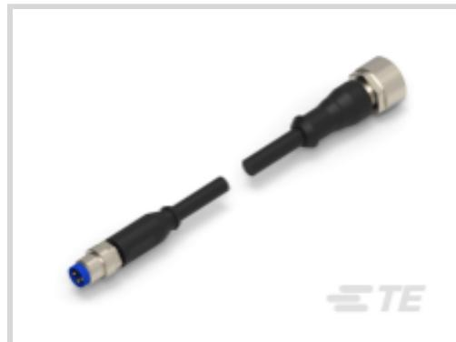
M8/M12 Application Type: **Sensor/Actuator**Number of Positions: **4**Connector & Keying Code: **A**Connector Type (End A): **M8 Plug**Connector Type (End B): **M12 Socket**[All M8 MS - M12 FS CABLE ASSY BL \(19\)](#)
