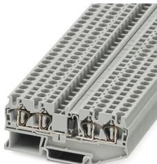
Component terminal block, with integrated diode 1N 5408, nom. voltage: 800 V, nominal current: 1.5 A, number of connections: 4, connection method: Spring-cage connection, Rated cross section: 1 mm<sup>2</sup>, cross section: 0.08 mm<sup>2</sup> - 6 mm<sup>2</sup>, mounting type: NS 35/7,5, NS 35/15, color: gray
