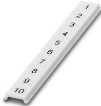
Zack Marker strip, flat, Strip, white, labeled, Printed vertically: consecutive numbers 1 ... 10, 11 ... 20, etc. up to 91 ... 100, mounting type: snapped, for terminal block width: 5 mm, lettering field size: 5.15 x 5.15 mm, Number of individual labels: 10
