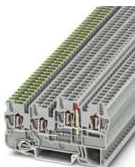
Installation ground terminal block, nom. voltage: 24 V, nominal current: 18 A, number of connections: 4, connection method: Spring-cage connection, Rated cross section: 2.5 mm<sup>2</sup>, cross section: 0.08 mm<sup>2</sup> - 4 mm<sup>2</sup>, mounting type: NS 35/7,5, NS 35/15, color: gray
