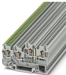
Installation ground terminal block, nom. voltage: 24 V, nominal current: 18 A, number of connections: 4, connection method: Spring-cage connection, Rated cross section: 2.5 mm<sup>2</sup>, cross section: 0.08 mm<sup>2</sup> - 4 mm<sup>2</sup>, mounting type: NS 35/7,5, NS 35/15, color: gray
