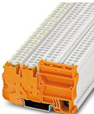
Installation ground terminal block, nom. voltage: 250 V, nominal current: 30 A, number of connections: 4, connection method: Spring-cage connection, Rated cross section: 2.5 mm<sup>2</sup>, cross section: 0.08 mm<sup>2</sup> - 4 mm<sup>2</sup>, mounting type: NS 35/7,5, NS 35/15, color: orange
