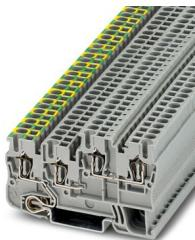
Installation ground terminal block, nom. voltage: 250 V, nominal current: 18 A, number of connections: 4, connection method: Spring-cage connection, Rated cross section: 2.5 mm<sup>2</sup>, cross section: 0.08 mm<sup>2</sup> - 4 mm<sup>2</sup>, mounting type: NS 35/7,5, NS 35/15, color: gray
