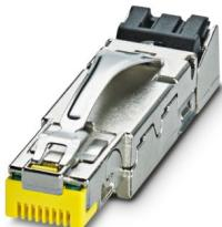
RJ45 connector, design: RJ45, degree of protection: IP20, number of positions: 8, 10 Gbps, CAT6<sub>A</sub>, material: Metal, connection method: Insulation displacement connection, connection cross section: AWG 26- 24, cable outlet: straight, color: yellow, Ethernet
