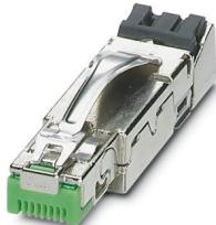
RJ45 connector, design: RJ45, degree of protection: IP20, number of positions: 8, 1 Gbps, CAT5, material: Metal, connection method: Insulation displacement connection, connection cross section: AWG 23- 22, cable outlet: straight, color: green, Ethernet/PROFINET
