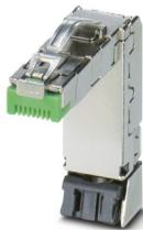
RJ45 connector, design: RJ45, degree of protection: IP20, number of positions: 6, 100 Mbps, CAT5 (IEC 11801:2002), material: Metal, connection method: Insulation displacement connection, connection cross section: AWG 26- 24, cable outlet: angled, High degree of resistance to vibration; 360° shielding; one-piece design; special tool-free assembly, VARAN
