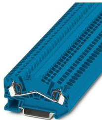
Feed-through terminal block, nom. voltage: 800 V, nominal current: 32 A, number of connections: 2, connection method: Spring-cage connection, 1 level, Rated cross section: 4 mm<sup>2</sup>, cross section: 0.08 mm<sup>2</sup> - 6 mm<sup>2</sup>, mounting type: NS 35/7,5, NS 35/15, color: blue
