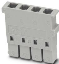
Connector housing, nom. voltage: 250 V, nominal current: 10 A, number of connections: 4, number of positions: 4, connection method: Crimp connection, Rated cross section: 1.5 mm<sup>2</sup>, cross section: 0.5 mm<sup>2</sup> - 2.5 mm<sup>2</sup>, mounting type: Plug-in mounting, color: gray
