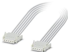
Assembled PCB connector / Connecting cable with 2 printed circuit board connectors, rated current: 6 A, cable length: Free input (0.1 ... 3.0 m), Head 1: 6-position, pitch: 2.5 mm, Crimp connection, Socket, Color: white, Cable type:Individual litz wire, PVC, 22 AWG, white, Head 2: 6-position, pitch: 2.5 mm, Crimp connection, Socket, Color: white, Cable type:Individual litz wire, PVC, 20 AWG, white, Individual litz wire, PVC, 22 AWG, white
