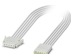
Assembled PCB connector / Connecting cable with 2 printed circuit board connectors, rated current: 6 A, cable length: Free input (0.1 ... 3.0 m), Head 1: 6-position, pitch: 2.5 mm, Crimp connection, Socket, Color: white, Cable type:Individual litz wire, PVC, 22 AWG, white, Head 2: 6-position, pitch: 2.5 mm, Crimp connection, Pin, Color: white, Cable type:Individual litz wire, PVC, 20 AWG, white, Individual litz wire, PVC, 22 AWG, white
