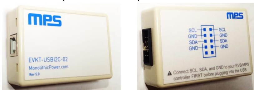
Figure 4: USB-to-I 2 C Communication Kit
