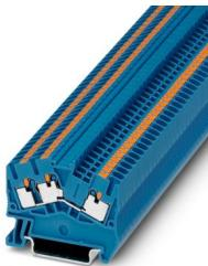
Feed-through terminal block, nom. voltage: 800 V, nominal current: 24 A, number of connections: 3, connection method: Push-in connection, 1 level, Rated cross section: 2.5 mm<sup>2</sup>, cross section: 0.14 mm<sup>2</sup> - 4 mm<sup>2</sup>, mounting type: NS 35/7,5, NS 35/15, color: blue
