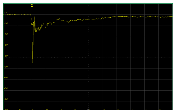
IEC 61000-4-2 -8 kV Contact ESD Clamping Voltage
