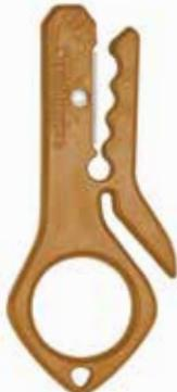
The key strip tool for twisted pair quickly strips outer cable jackets from CAT 3, 5, 5e and 6 data cable.
