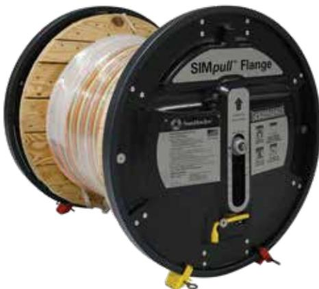
The **SIMpull™ Flange**'s patented shaft less design, safely allows one person to turn a wooden or plastic reel up to 34 in. and 2000 lbs into a time saving, field-installable solution that removes the need to handle heavy jack stands. Each flange rotates independently, and allows free movement of loaded wooden or plastic reels. The **SIMpull™ Flange** is reusable in the field and can be installed on multiple reels throughout the jobsite.
