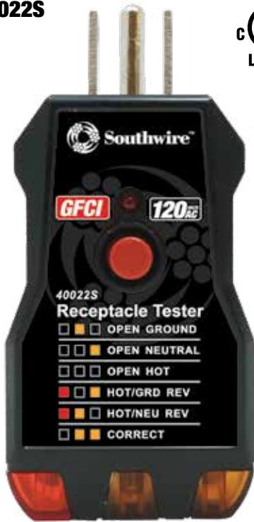
GFCI receptacle tester quickly identifies the most common wiring faults associated with 3-wire 120V outlets. Just plug it into the outlet and the indicator lights quickly tell you if the outlet is wired correctly. Press the red button to verify that a GFCI circuit is functioning properly.
