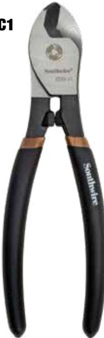
Many coax cables today have a copper clad steel (CCS) center conductor. This specially designed cutter is made to reliably cut CCS coax that might damage standard cable cutters.
