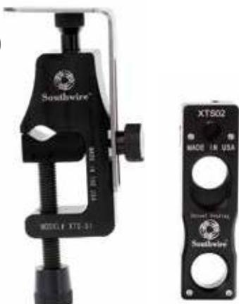
XTC100 Combination stripper kit includes XTS01 and XTS02. Strips wire and cable from #6 AWG-1000 KCMIL.
