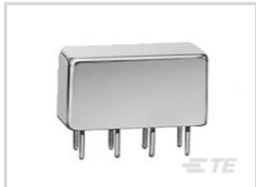
Contact Arrangement: **2 Form C, DPDT, 2 C/O**Input Voltage: **12 VDC**Contact Current Rating: **2 A**Coil Voltage Rating: **12 VDC**Coil Resistance: **310 Ω**
