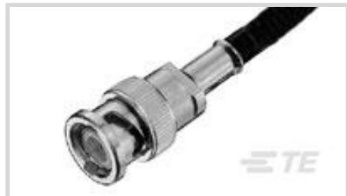
RF Interface: **BNC**RF Connector Style: **Plug**RF Connector Mated Outer Diameter (Approximate): **14.53 mm [ .572 in ]**Impedance: **50 Ω**Compatible With RF Cable Type: **RG 142, RG 142A, RG 142B**[All BNC RF Connector: Plug Kit, Straight, 4 GHz, Military Grade \(0\)](#)
