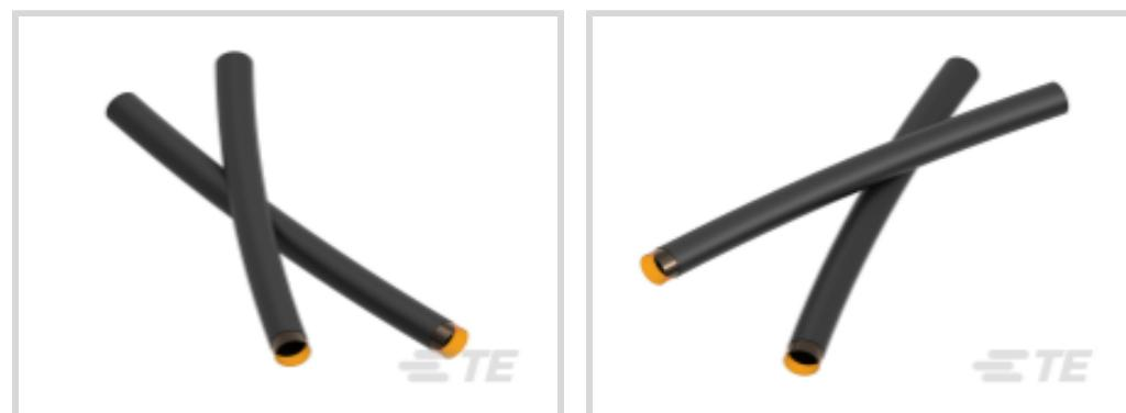
Primary Product Color: **Black**Wall Type: **Dual Wall**Expanded Inside Diameter (Min): **25.4 mm [ 1 in ]**Recovered Inside Diameter (Max): **12.7 mm [ .5 in ]**Shrink Ratio: **2:1**[All TAT-125 Heat Shrink Tubing \(71\)](#)
