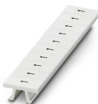
Zack marker strip, Strip, white, labeled, can be labeled with: CMS-P1-PLOTTER, printed horizontally: Identical numbers 1 or 2, etc. up to 100, mounting type: snapped, for terminal block width: 5.2 mm, lettering field size: 5.15 x 10.5 mm, Number of individual labels: 10
