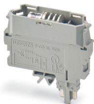
Component connector, specifically for holding the SKN 2,5 diode, nom. voltage: 400 V, nominal current: 10 A, connection method: Plug-in connection, depth: 37.5 mm, width: 12.3 mm, height: 41.2 mm, number of positions: 1, color: gray, mounting type: Pluggable (slot)
