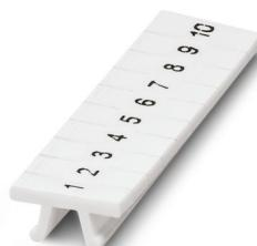
Zack marker strip, Strip, white, labeled, printed horizontally: consecutive numbers 1 ... 10, 11 ... 20, etc. up to 91 ... 100, mounting type: snapped, for terminal block width: 3.5 mm, lettering field size: 3.5 x 10.5 mm, Number of individual labels: 10
