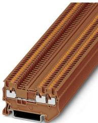
Feed-through terminal block, nom. voltage: 500 V, nominal current: 17.5 A, number of connections: 3, connection method: Push-in connection, 1 level, Rated cross section: 1.5 mm<sup>2</sup>, cross section: 0.14 mm<sup>2</sup> - 1.5 mm<sup>2</sup>, mounting type: NS 35/7,5, NS 35/15, color: brown
