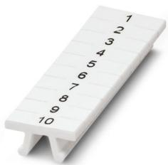
Zack marker strip, Strip, white, labeled, Printed vertically: consecutive numbers 1 ... 10, 11 ... 20, etc. up to 91 ... 100, mounting type: snapped, for terminal block width: 3.5 mm, lettering field size: 3.5 x 10.5 mm, Number of individual labels: 10
