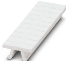
Zack marker strip, Strip, white, unlabeled, can be labeled with: PLOTMARK, CMS-P1-PLOTTER, mounting type: snapped, for terminal block width: 3.5 mm, lettering field size: 3.5 x 10.5 mm, Number of individual labels: 10
