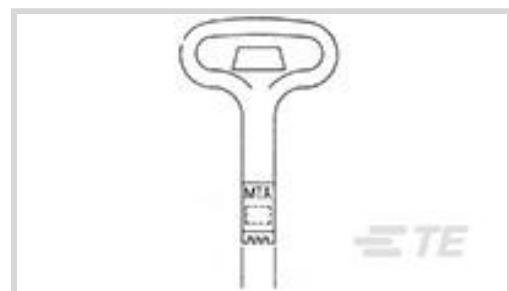
Insertion & Extraction Tool Application: **Contact-to-Wire**
