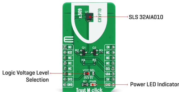
Trust M Click comes with up to 10kB user memory that can be used to store X.509 certificates and data. OPTIGA™ Trust M1 is based on Common Criteria (CC) Certified EAL6+ (high) hardware enabling it to prevent physical attacks on the device itself and providing high assurance that the keys or arbitrary data stored cannot be accessed by an unauthorized entity.
