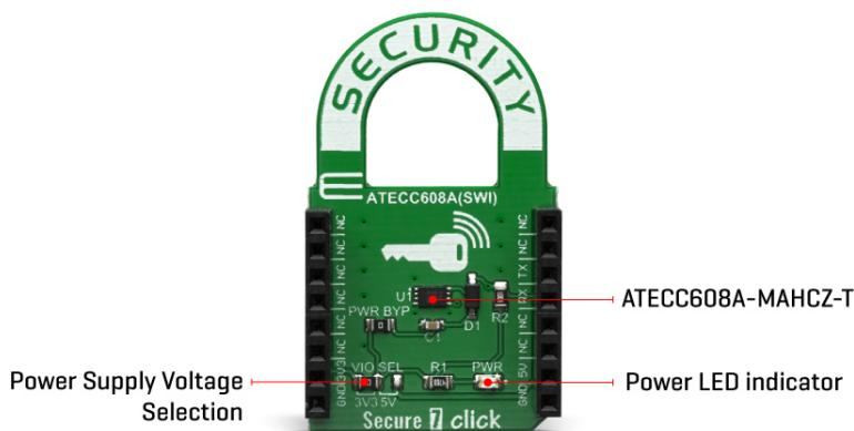
It features a wide array of defense mechanisms specifically designed to prevent physical attacks on the device itself, or logical attacks on the data transmitted between the device and the system. Hardware restrictions on the ways in which keys are used or generated provide further defense against certain styles of attack.
