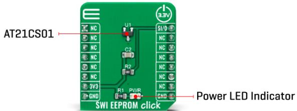
The AT21CS01 benefit from 100 years of data retention, combining their unprecedented data storage with excellent energy efficiency. It is characterized by high reliability and ultra-high writing endurance capability, allowing more than one million cycles for each memory location to meet today's high-write endurance applications' requirements.
