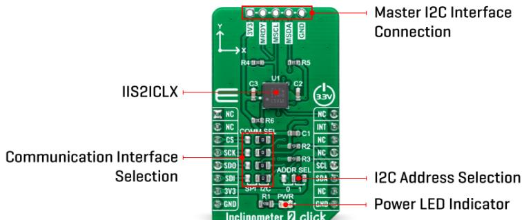
The IIS2ICLX has an unmatched set of embedded features (programmable FSM, Machine Learning Core, sensor hub, FIFO, event decoding, and interrupts) and delivers high accuracy and performance at low power. The sensing element is manufactured using a dedicated micromachining process developed by STMicroelectronics to produce inertial sensors and actuators on silicon wafers.
