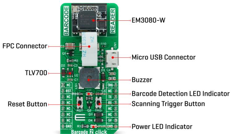
The EM3080-W scanner module uses a flat cable to connect to the Click board™, via the FPC Connector which is located on the top side of the PCB. This flat cable carries all the signals used in communication between the EM3080-W module and the host MCU, such as the RX, TX, buzzer, USB, LED, reset, and scanning trigger lines.
