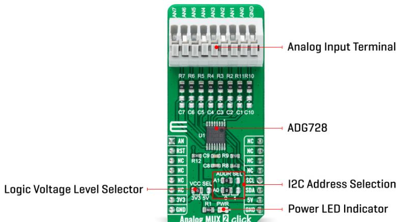
Each bit of the 8-bit serial word corresponds to one switch of the device. Internal switching channels are independently controlled by an individual bit, providing an option of having any, all, or none of the switches activated. All of the input channels of the multiplexer can be easily connected to a 9 pole spring action block terminal, without having to use any additional tools, such as screwdrivers, while the output pin from the multiplexer is routed to the AN pin on the mikroBUS™ socket.
