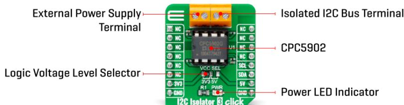
This optically coupled I2C bus repeater is ideal for Power-over-Ethernet (PoE) applications, providing buffering and isolation of the clock and data signals between the host controller and the Power Supply Equipment (PSE) controller. Additional applications include power supply high side interface, I2C bus length extender, and isolated signal monitoring and control. An extensive operational power supply range of 2.7V to 5.5V also enables I2C logic level translation applications.
