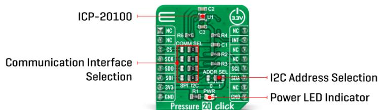
This MEMS sensor consists of a capacitive pressure sensor whose capacitance changes according to the pressure applied. An integrated temperature sensor on the same MEMS sensor allows accurate temperature measurements. Other industry-leading features include up to 20-bits output data, programmable digital filters, calibration, FIFO, and programmable interrupts.
