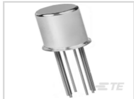
Contact Arrangement: **2 Form C, DPDT, 2 C/O**Input Voltage: **26.5 VDC**Coil Voltage Rating: **26.5 VDC**Coil Resistance: **1560 Ω**Coil Power Rating DC: **450 mW**
