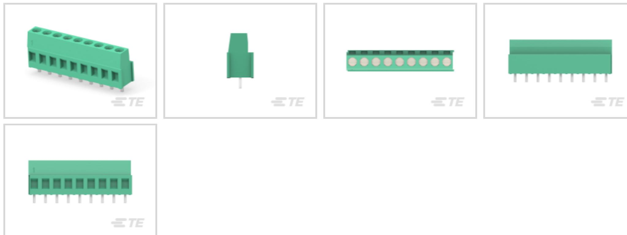
Terminal Block Connector Type: **Header**Connector System: **Wire-to-Board**Number of Positions: **9**Centerline (Pitch): **5 mm [.197 in]**Number of Rows: **1**
