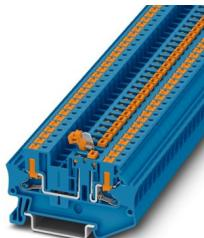
Knife-disconnect terminal block, nom. voltage: 500 V, nominal current: 20 A, 1 level, connection method: Push-in connection, Rated cross section: 4 mm<sup>2</sup>, cross section: 0.2 mm<sup>2</sup> - 6 mm<sup>2</sup>, mounting: NS 35/7,5, NS 35/15, color: blue
