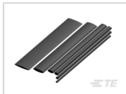
Primary Product Color: **Black**Wall Type: **Single Wall**Expanded Inside Diameter (Min): **43.18 mm [ 1.7 in ]**Recovered Inside Diameter (Max): **12.7 mm [ .5 in ]**Shrink Ratio: **3:1**[All SST-FR Heat Shrink Tubing \(46\)](#)
