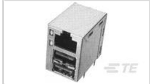
Port Matrix Configuration: **2x1**Port Configuration: **Single Port**Modular Jack & Plug Interface Type: **RJ45 over Dual USB**Connector Profile: **Low**Modular Jacks & Plugs Products: **Combo Jacks**
