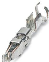
Female contact, is inserted into the plug after crimping the conductor, for the module plug housing MCC 1...-STZ-3,81 and MCC 1...--STZF-3,81, for cross sections of 0.5 mm<sup>2</sup> to 1 mm<sup>2</sup>
