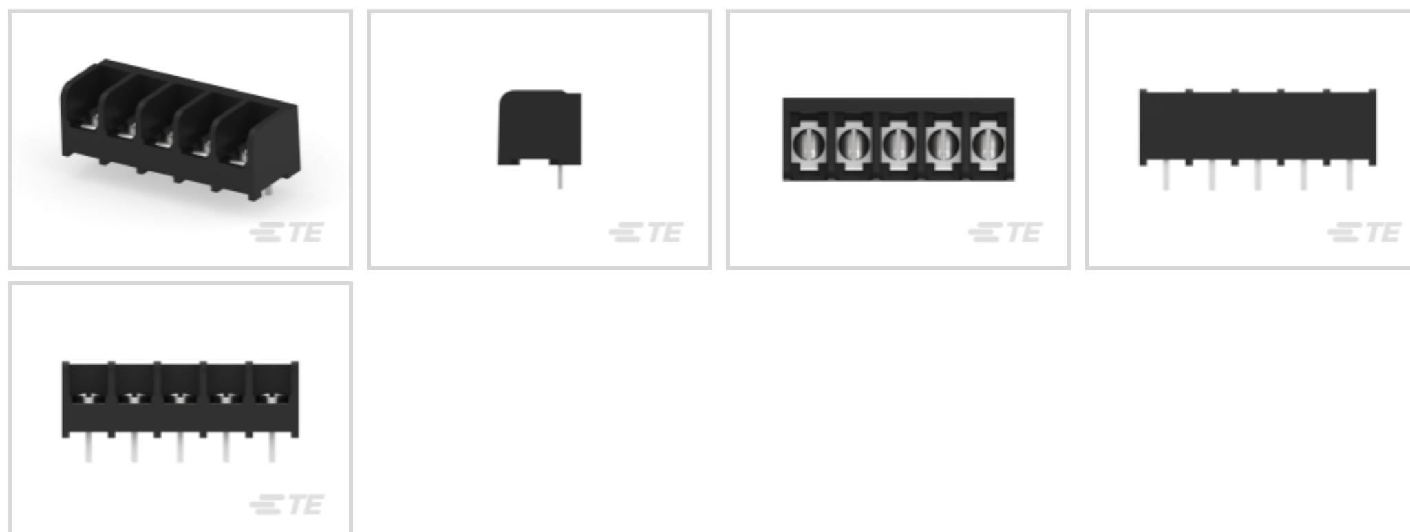
Barrier Strip Style: **Tri-Barrier**Bottom Termination Type: **Printed Circuit Pin**Connector System: **Wire-to-Board**Number of Positions: **5**Centerline (Pitch): **9.53 mm [.375 in]**
