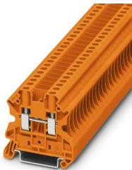
Feed-through terminal block, With breakout partition plate in the bridge shaft, nom. voltage: 1000 V, nominal current: 32 A, number of connections: 2, number of positions: 1, connection method: Screw connection, Rated cross section: 4 mm<sup>2</sup>, cross section: 0.14 mm<sup>2</sup> - 6 mm<sup>2</sup>, mounting type: NS 35/7,5, NS 35/15, color: orange
