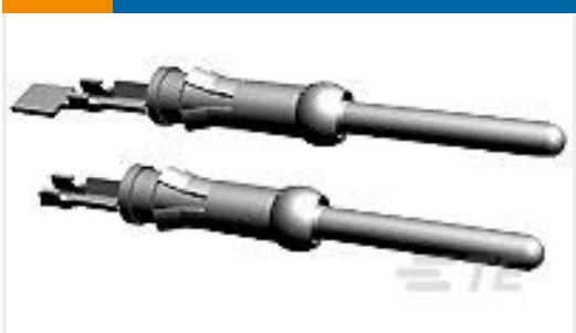
TE Part # 66564-8 III+ PIN,24-20,30AU/FL,STRIP
