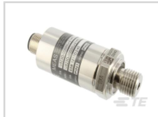
Pressure Sensor Type: **Industrial Pressure Transducer**Pressure: **.14 bar [ 2.03 psi ]**Pressure Type: **Absolute**Supply Voltage Range: **9 - 30 V**Output Signal Type: **4 - 20 mA**
