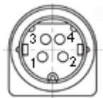
PINS 2,4: +V, PINS 1, 3, SHELL: COM (and EARTH GROUND if power supply grounding configuration specifies grounded Common return)
